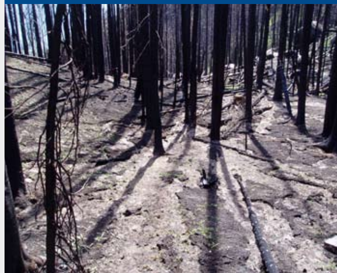
Evidence of concentration of overland flow on water-repellent soils. Kuskonook Creek drainage, August 2004.
